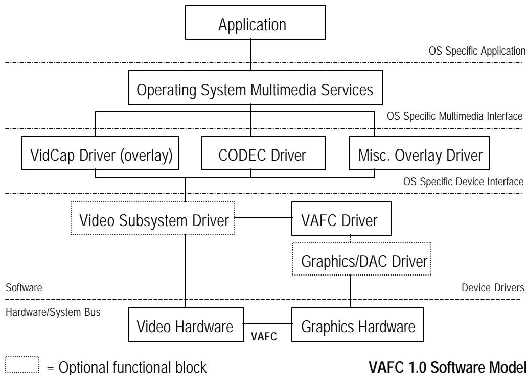
The video subsystem has various system drivers that can exploit the VAFC interface, and some applications which do not fit into the current architecture of MCIAVI also might want to use this resource. These drivers/custom applications (here on specified as *drivers*) are required to open the VAFC driver, communicate with the driver through the standard driver message interface to configure it for the best performance, and close the driver when the driver has finished using the VAFC bus.
