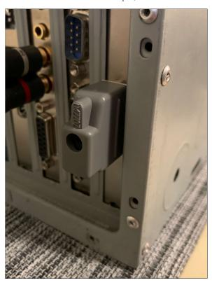
If your VGA adapter provides color output even without the terminator dongle, or you want to use the VGA output for other purpose, then you can just leave the dongle in the box.
