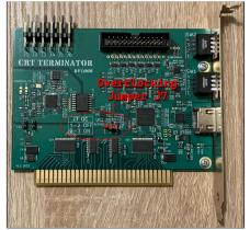
Jumper settings J3-6 enable manually configuring the appropriate video signal sampling phases to use. In order for these jumpers to take effect, jumper J2 must first be set to state 2-3.
