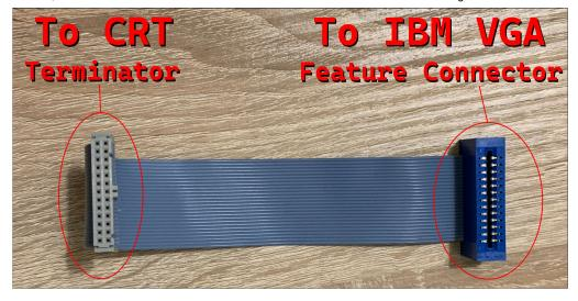
Connecting the cable to the CRT Terminator end is easy, because there is only one orientation that the cable fits. This orientation identifies which side of the cable will be Pin 1:
