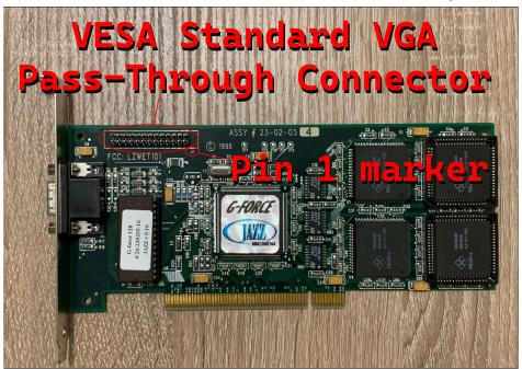
Use the following video cable to connect CRT Terminator to your VGA adapter with a VSVPC connector:
