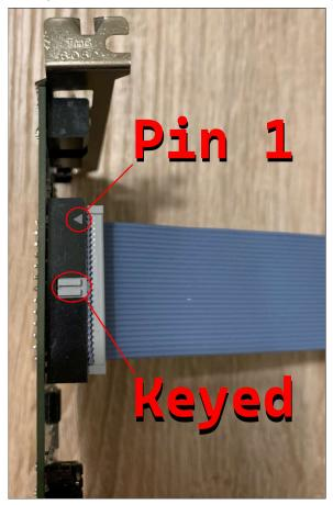
Note that the 2x13 pin VSVPC connector on the VGA adapter is <u>unkeyed</u>. That is, it is possible to connect the video cable to this connector incorrectly, rotated 180 degrees.
