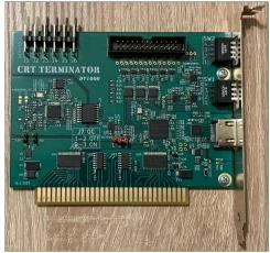
This VGA Feature Connector bus bypasses the signal degrading digital-to-analog video conversion step (RAMDAC), and enables CRT Terminator to output a fully digital video signal. CRT Terminator converts and upscales this 8-bit palettized digital video into a True Color 24-bit RGB DVI-D output stream that is compatible with HD video on modern flat panel displays.
