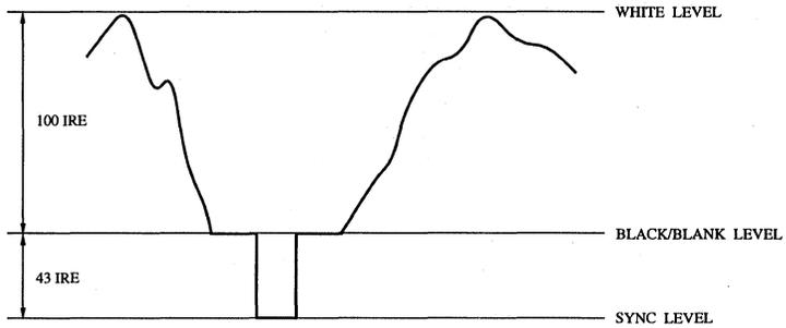
Note: 75 Ω doubly-terminated load and SETUP = 0 IRE. VREF = 1.235 V and RSET = 147 Ω. RS-343A levels and tolerances are assumed on all levels.
