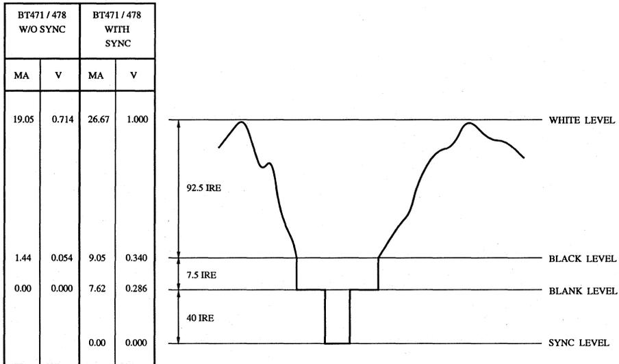
Note: 75 Ω doubly-terminated load and SETUP = 7.5 IRE. VREF = 1.235 V and RSET = 147 Ω. RS-343A levels and tolerances are assumed on all levels.
